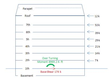
Comparing the over turning moments for both wind and seismic, seismic caused a greater over turning moment than wind. Thus, 1.2D + 1.0E + L + 0.2S is the governing load combination for strength design as compared with 0.9D + 1.0E + 1.6H.
