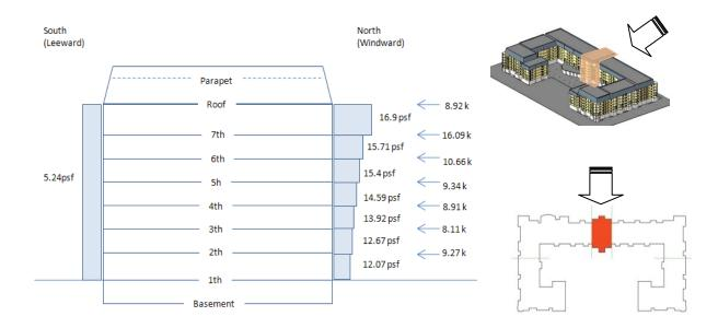
The wind loads were recalculated because of a discrepancy in assigning the floor heights in Technical Report 3.
