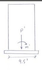
Resisting Moment =  $P'(\frac{q.5}{2})$   $M_{resisting} = 7351.5^{k}(\frac{q.5}{2}) = 11169.63^{lk}$  $M_{resisting} = 11169.63 > 8474.87^{lk}$  ok V
