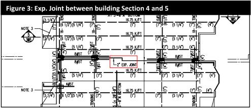
Recently, it was discovered that a double column (12" x 30") is placed back to back, one on each side of an expansion joint.
